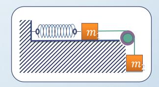
Example: A 2.0 kg block slides along a floor with speed  $v_1 = 4.0$  m/s. It then runs into and compresses a spring, until the block momentarily stops. Its path to the initially relaxed spring is frictionless, but as it compresses the spring, a kinetic frictional force of magnitude 15 N acts on it. The spring constant is 10,000 N/m. By what distance d is the spring compressed when the package stops?
