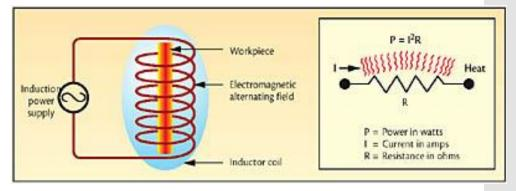
The induced current in a metal plate is named the eddy currents.
