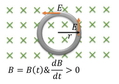
Here the induced electric field is uniformly distributed in the circular wire (rather than in a certain length of wire).
