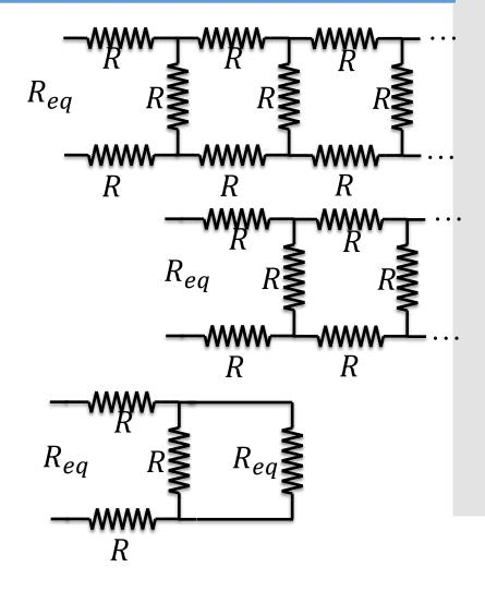
$$R_{eq} = R_T + \frac{1}{\frac{1}{R_L} + \frac{1}{R_{eq}}}$$
