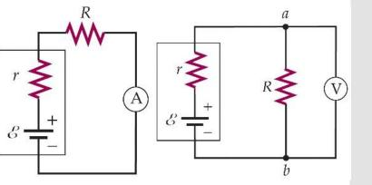
Internal Resistor in The Battery
