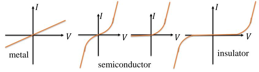
Metals show a linear I-V behavior whereas insulators show a nonlinear behavior, temperature coefficient of resistivity (TCR):  $\frac{1}{\rho} \frac{d\rho}{dT}$
