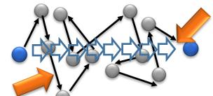
drift velocity, driven by electric field
