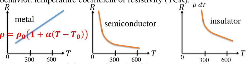
Resistance of metals increase linearly with temperature whereas that of insulators decrease exponentially with temperature.
