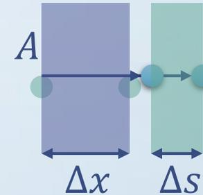
$$B = \frac{\text{volume stress}}{\text{volume strain}} = -\frac{\Delta F/A}{\Delta V/V} \quad \text{Bulk modulus: } \Delta P = -B \frac{\Delta V}{V} = -B \frac{A\Delta s}{A\Delta x}$$
