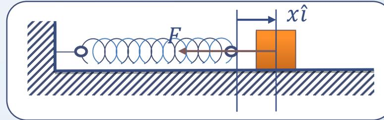
Newton's 2<sup>nd</sup> Law, the block of mass  $m$  is reacting to the external, restoring force by the spring.
