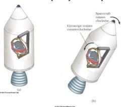
The motion of gyroscope and the conservation of angular momentum are applied in finding the direction for space travel.
